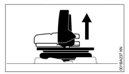
► Remove the tank cap.
