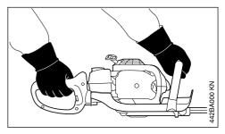
Right hand on the control handle and left hand on the handlebar
