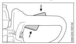
Press down the throttle trigger lockout and open the throttle – the choke knob moves to the run position <u>-</u>. After a cold start, warm up the engine by opening the throttle several times
