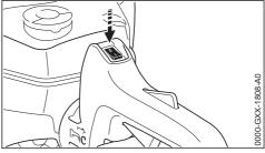
Move the stop switch in the direction of 0 – when released, the stop switch springs back to the normal run position I.
