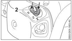
► Depress the outer ring (arrows) of the choke knob (2) and then turn it to  $\overline{f}$ .
