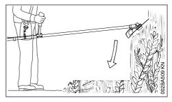
To cut wild growth and scrub, lower the brush knife down onto the growth to achieve a shredding effect – always keep the cutting attachment below hip level during this process.
