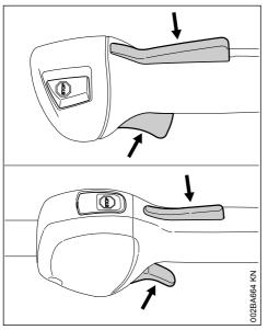
Press down the throttle trigger lockout and open the throttle – the choke knob moves to the run position I. After a cold start, warm up the engine by opening the throttle several times.
